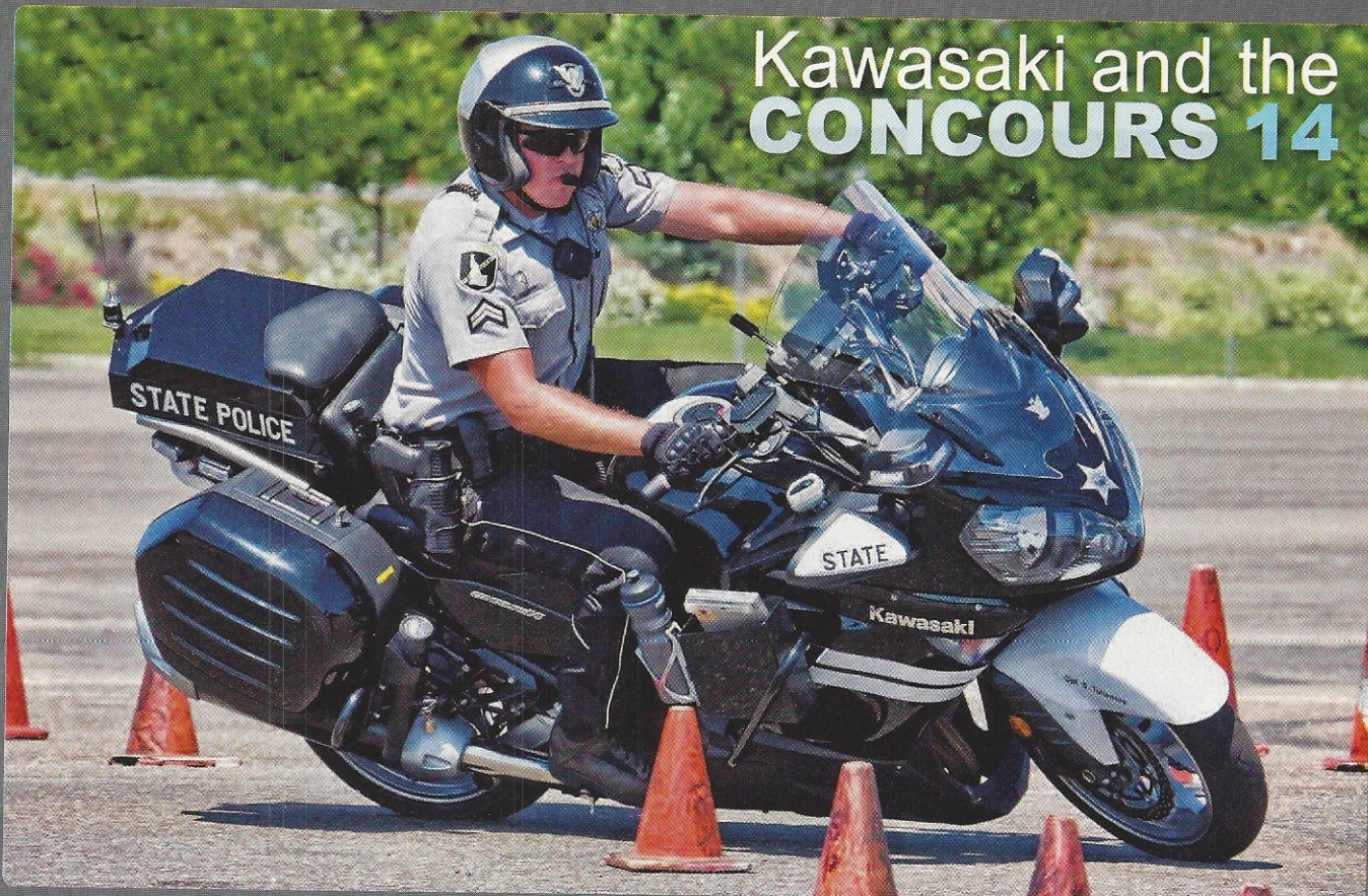
Corporal Scott Tulleners is shown riding the Concours 14, which has ABS. Also, the front brakes use twin discs and four piston calipers.
